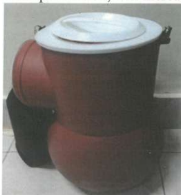
Fig. 1 Developed Neera Collector
